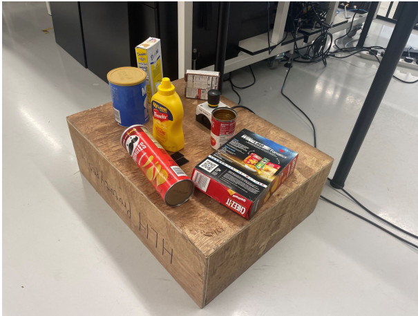
Fig. 7: In this image, we illustrate the setup of the first operational scenario, where the robot reaches a button in a cluttered environment. The button is placed on a base that obstructs the view from the robot's camera
